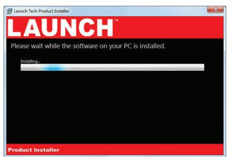
4. Once the setup application has finished, Connect the USB cable to your J-Box 3 and to the PC. Once you have gotten a message in the lower right hand corner that the device has been installed, click Activate My device. Then Click Exit.
